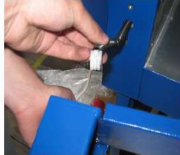
picture 5: putting throw belt motor connector
