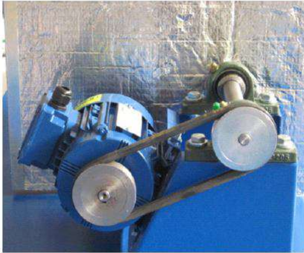
picture 17: belt transmission view
