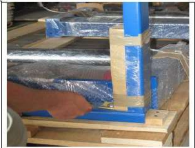
picture 4: loosening locking screws
