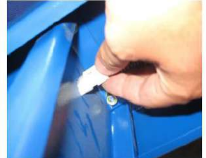
picture 6: connecting belt motor connector
