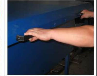
picture 9: sliding on side top cover
