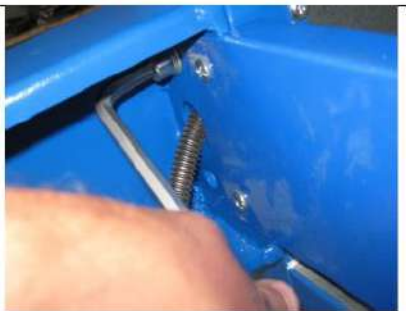
picture 10: locking inlet/outlet screws
